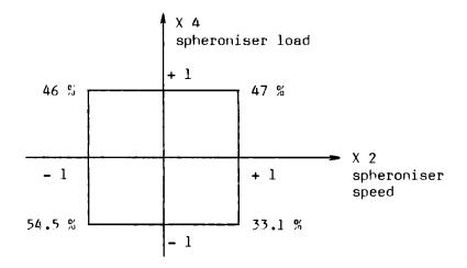
The negative effect of spheroniser speed is important only at the lower load.
