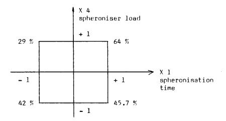
The effect of increased spheronisation time is demonstrated at higher load (4 kg) but not at the lower value (1 kg).
